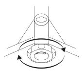
◆ To decrease the blade angle, turn the twist pitch knob counterclockwise.
