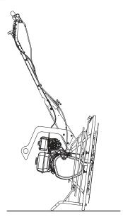
*NOTICE* Do not tilt the machine in any other direction. Incorrect tilting or leaning can cause problems with engine oil pouring out through the valve into the carburettor.
